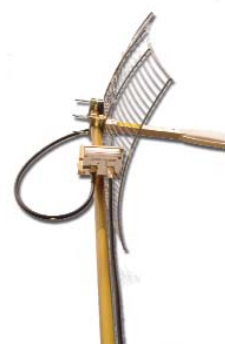
The A2440-RF amplifier mounted on a pole next to a grid dish antenna.
