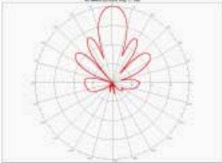
Azimuth Radiation Pattern Midband Freq. 3.7GHz
