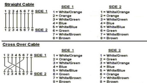
Figure A-1 Straight-Through and Crossover Cable
